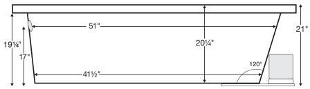
IMPORTANT: Air baths and tubs with a pre-leveled foam base or frame system add 2-3" to overall tub height.
